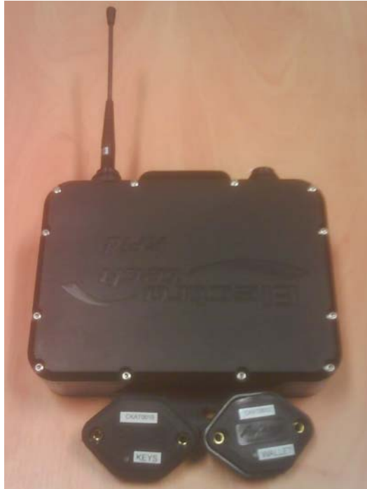
Figure 8: RFID reader and two 3D active tags.
