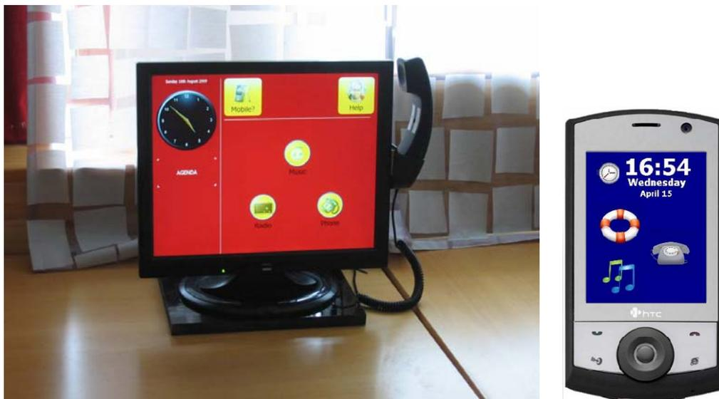
Figure 2. CHH touch screen with handset, CCA mobile device
